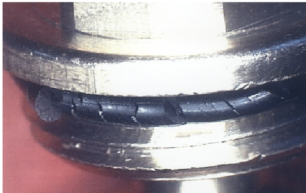
Figure 5 – failure cause: ozone cracks
