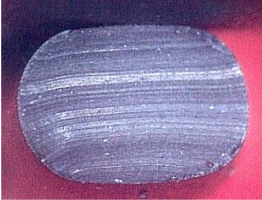
Photo 7: Permanently deformed O-Ring.
