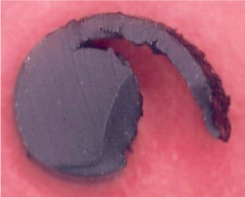
Photo 8: Extruded O-Ring (excessive seal gap)
