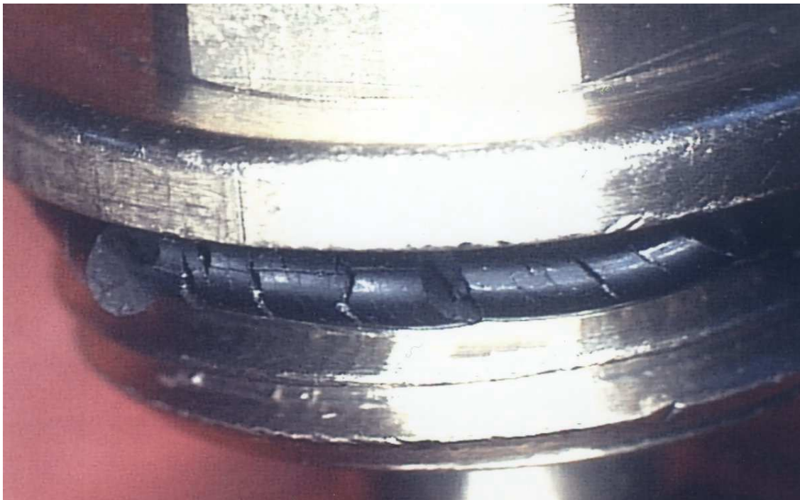
Photo 5: Ozone splits on an assembled o-ring on sub component following several weeks in storage without light and air protection.
