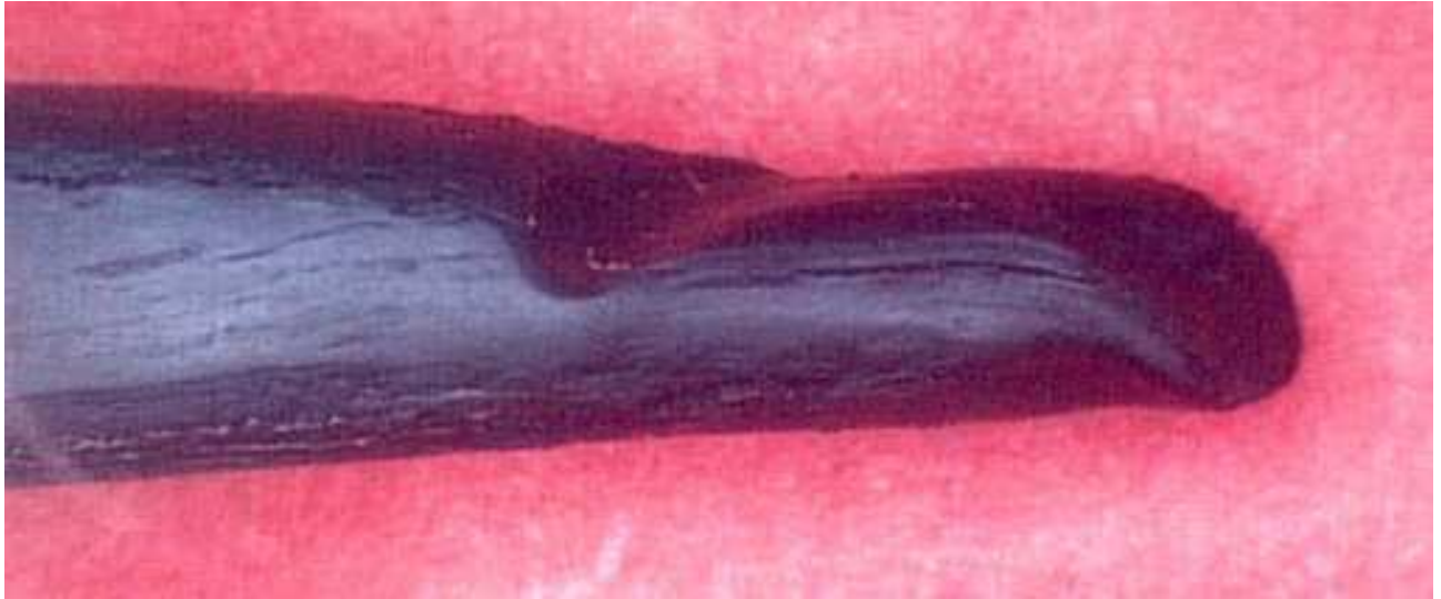
Photo 3: Sheared o-ring from passing over flow channel during assembly.
