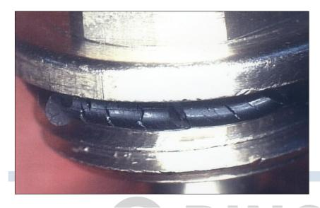
**Fig. 3:** Pre-assembled NBR O-ring, which after a few weeks of storage became very severely cracked
