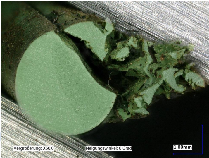
Figure 6: Strong swelling which resulted in shear
