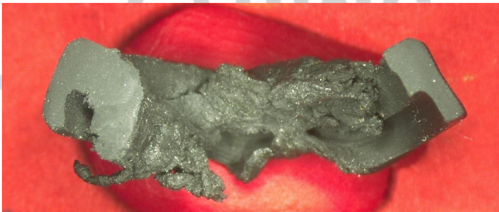
Figure 7: Strongly swelled EPDM-seal after dynamic stress of a lip seal
