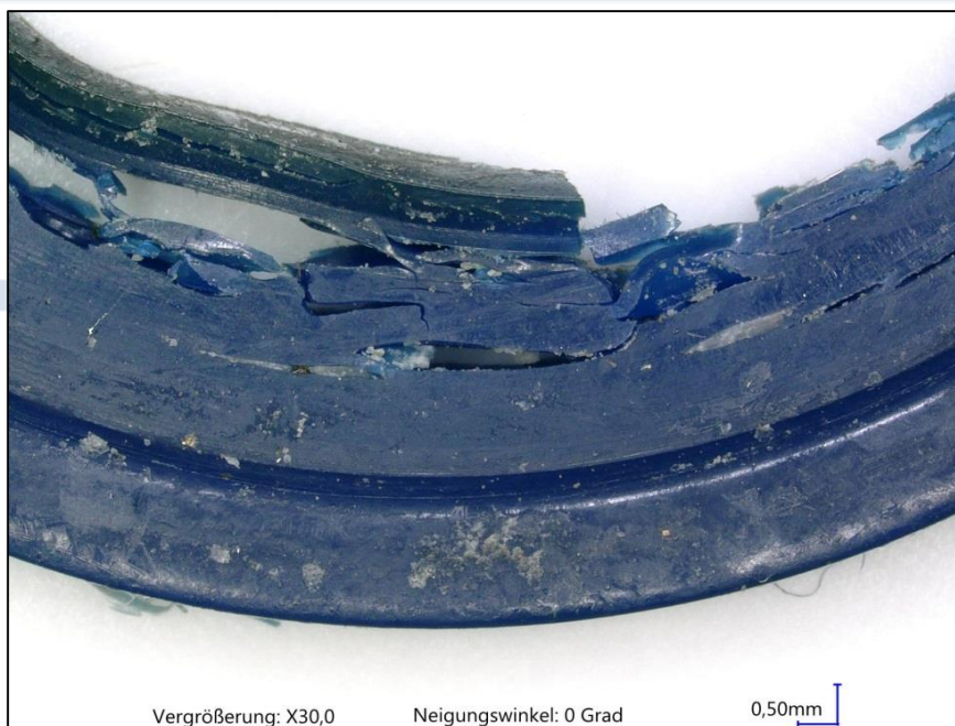
Figure 4: Hydrolysis (= chemical erosion by water) of a polyurethane seal
