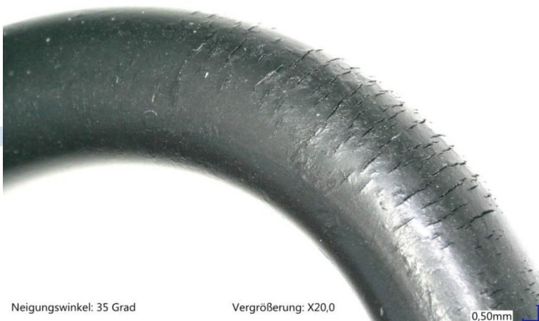
Fig. 18: Cracks caused by the post-processing step "post-curing" (local overheating due to defective or incorrectly set tempering furnace)
