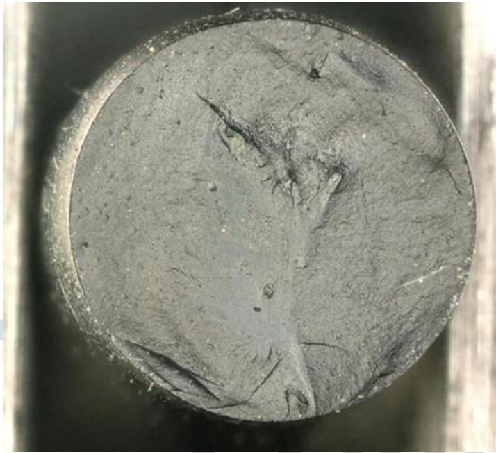
Fig. 5: Torn O-ring caused by a vulcanization error
