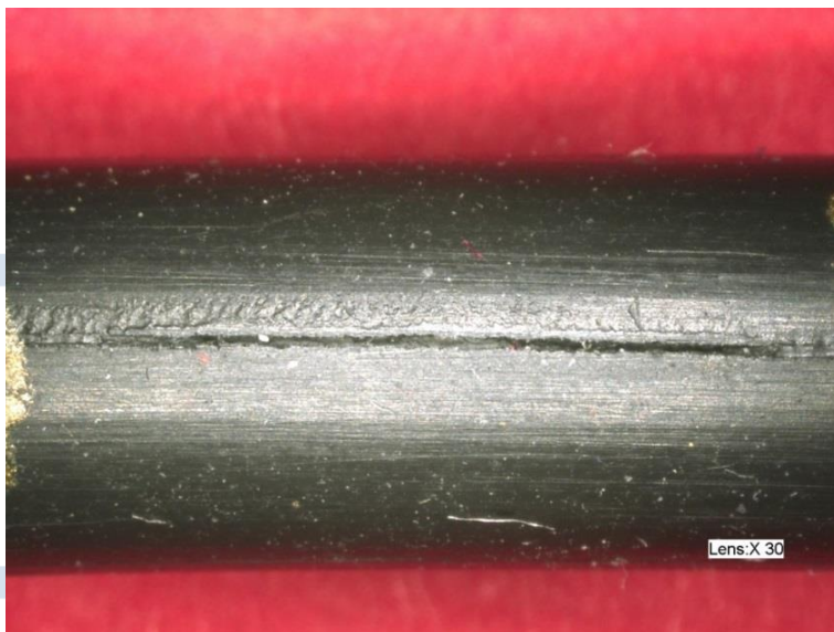
Fig. 12: Shrinkage crack on an O-ring
