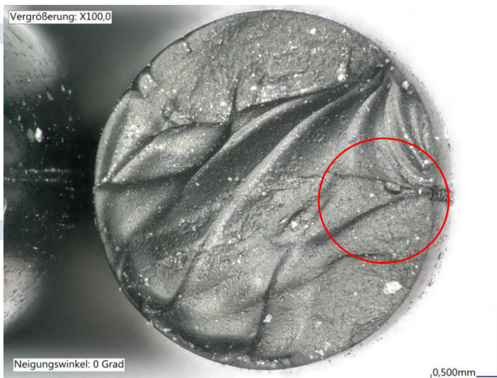
Fig. 6: Torn O-ring due to vulcanization defect: Inhomogeneous, fissured fracture surface
