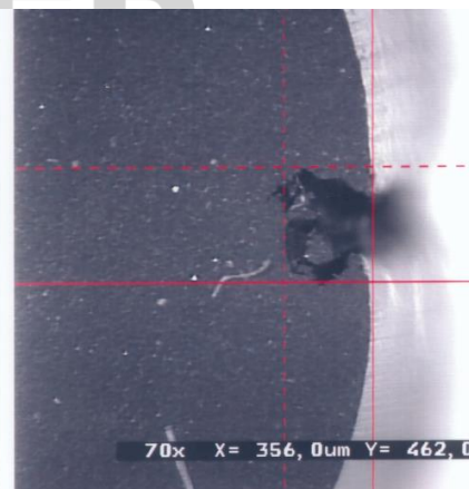
Figs. 13 and 14: Shrinkage cracks at the tool parting plane of an O-ring and on the right in a cross-cut O-ring
