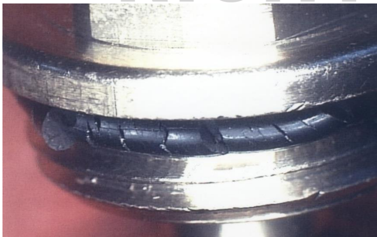
Fig. 19: Pre-assembled O-ring, which showed ozone cracks after several weeks due to the pre-stressing and ozone from the ambient air.
