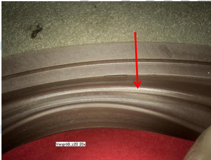
Fig. 15: Demolding crack on a molded gasket
