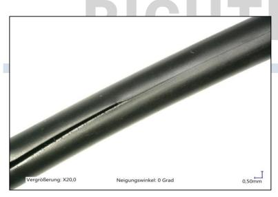
**Fig. 3:** Installation-related crack due to the effect of a sharp edge in the installation space
