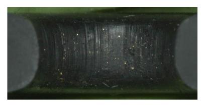
**Fig. 2:** Inside of a cut EPDM Oring from a thermostatic valve: Metal particles are clearly visible in the grooves (hydroabrasion).
