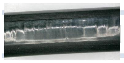
**Fig.3:** Abrasion of a "statically" used O-ring by axial stroke
