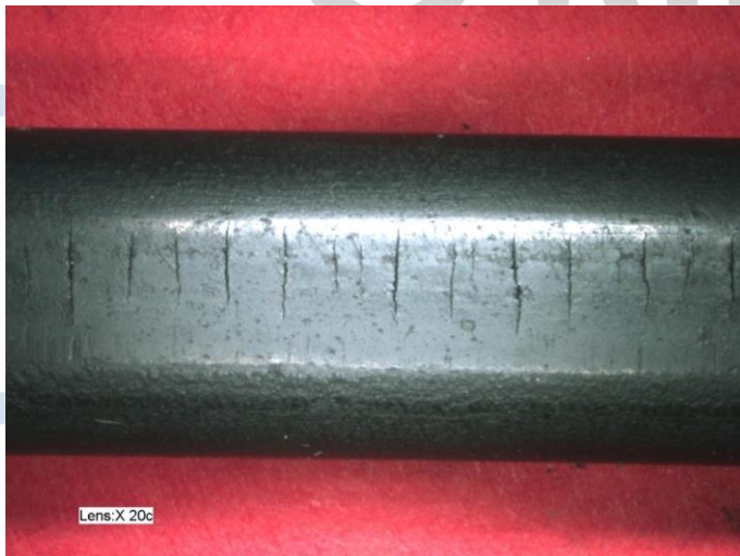
Figure 1: Thermally damaged O-Ring, fully cured, during bending cracks visible on contact surface
