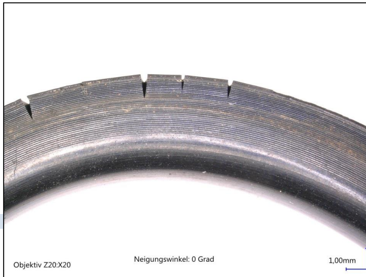
Figure 3: Brittle NBR O-ring shows cracks during bending (rotary scoring is an impression of the mating surface) Differentiation from ozone cracks: hardening of cracked zones. With ozone or fatigue cracking there are cracks in the still elastic elastomer matrix.
