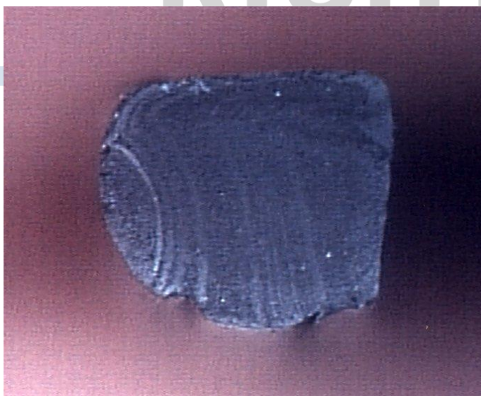
Figure 2: Cross section of severely overheated O-ring (short operating time) due to dry start-up of a slide ring seal compression set and the striking of local embrittlement, the core is still fully elastic
