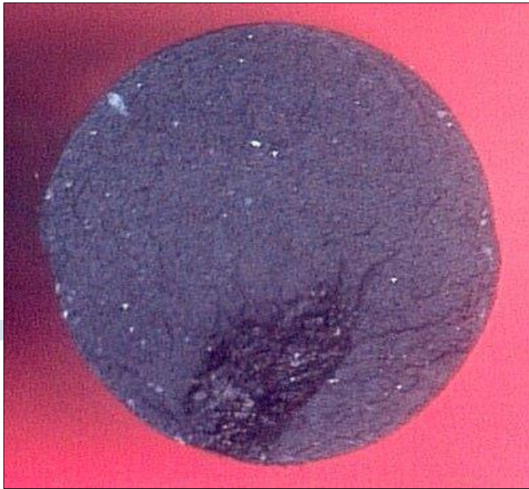
Fig. 2: Crack triggered by ingress of foreign material
