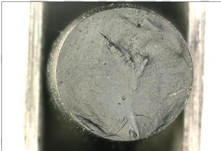
Fig. 1: Cracked O-ring caused by a vulcanization defect
