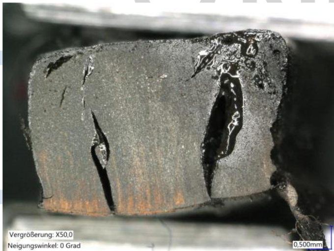
Fig. 4: Internal cracks due to explosive overheating or explosive evaporation
