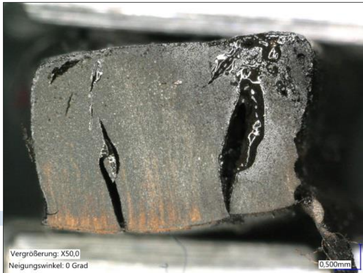
Fig. 3: Internal cracks due to explosive overheating or explosive evaporation
