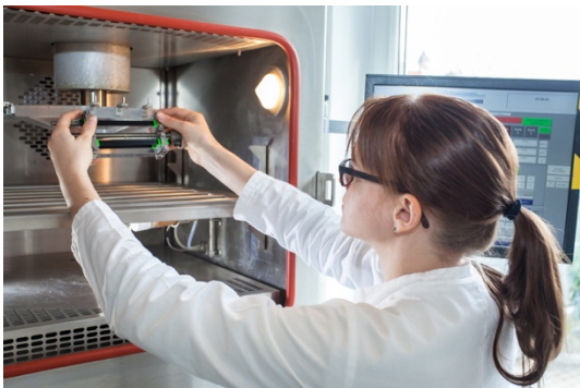
Figure 4: New in the testing laboratory since 2015 - ozone testing
