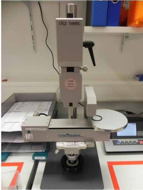
Fig. 1: Stationary IRHD micro-tester with laser-guided table for exact hardness measurement of O-rings (CM method)
