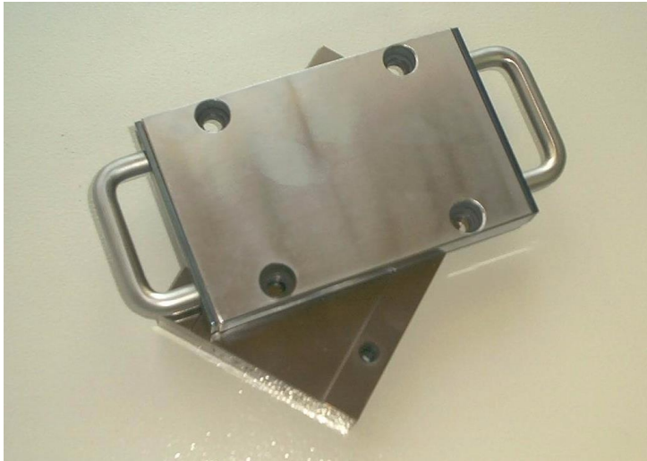
Fig.3: Compression set test tools with base plate ground to different depths (see lower plate), the use of spacers is not necessary.
