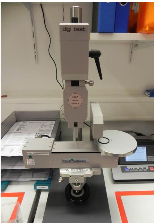
Fig. 2: One of two stationary IRHD, micro-testing devices in the O-ring testing laboratory Richter. They have a laser-guided bench, especially for the exact hardness measurement of O-rings.
