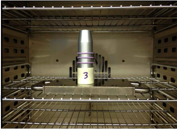
Fig. 3: Tensile Set on O-rings using a test mandrel in a laboratory furnace (radial elongation)
