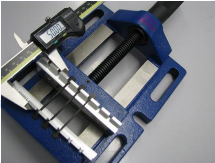
Fig 1: Tensile Set: standard test specimen in initial position, still relaxed state (50mm)
