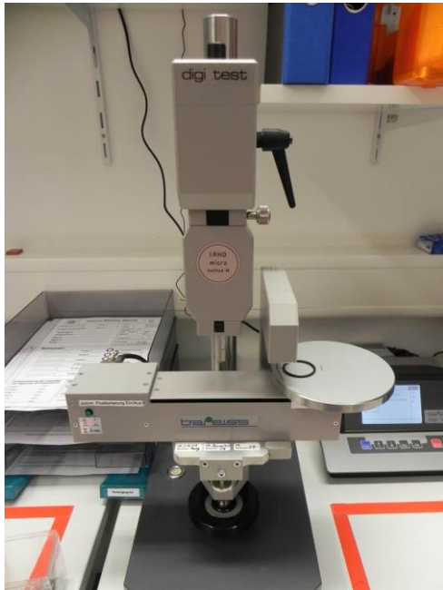
Fig. 1: Stationary IRHD micro-tester with laser-guided table for exact hardness measurement of O-rings (CM method)
