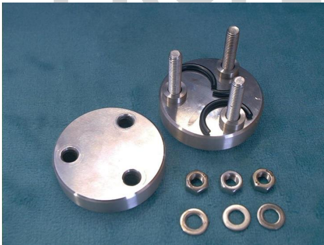
Fig. 4: Plane plates for compression set measurement with spacers: there are three O-ring sections on the base plate.
