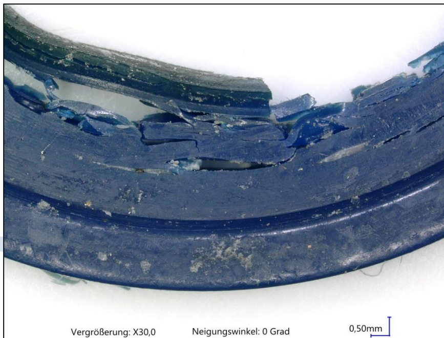
Figure 4: Hydrolysis (= chemical degradation by water) of a poly-urethane seal
