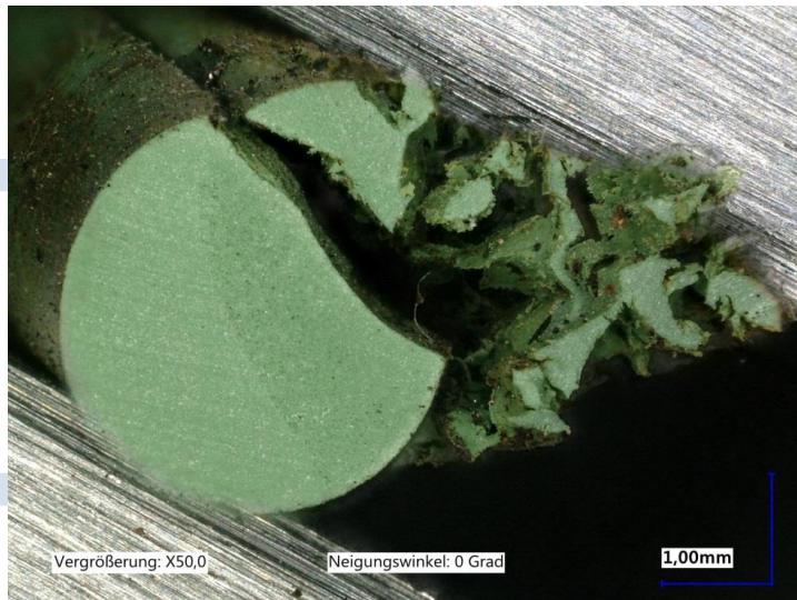
Figure 6: Strong swelling which resulted in shear
