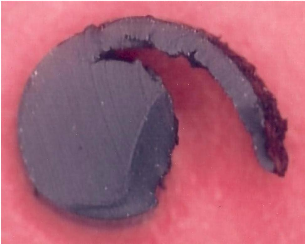
*Photo 8: Extruded O-Ring (excessive seal gap)*
