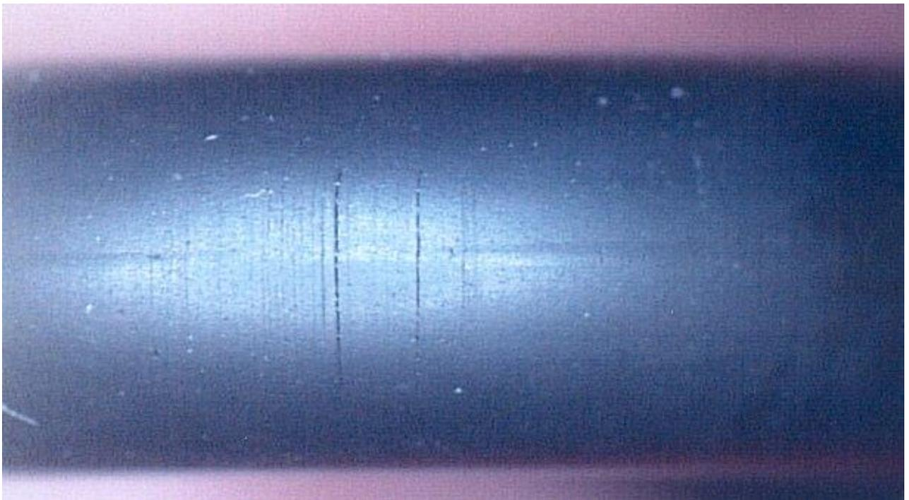
*Photo 4: O-Ring damage from passing over guide chamfer.*
