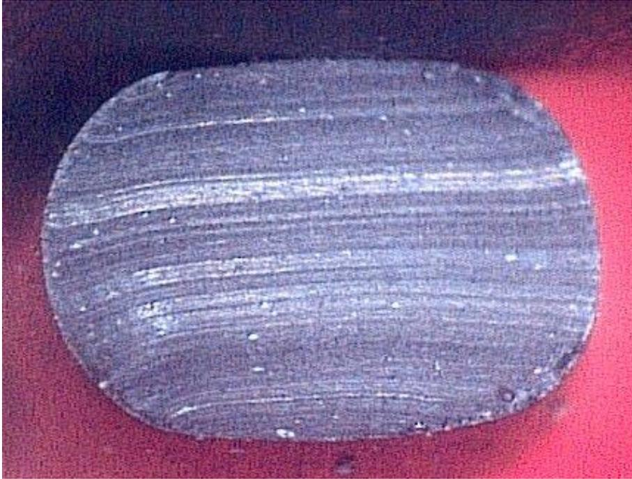
*Photo 7: Permanently deformed O-Ring.*
