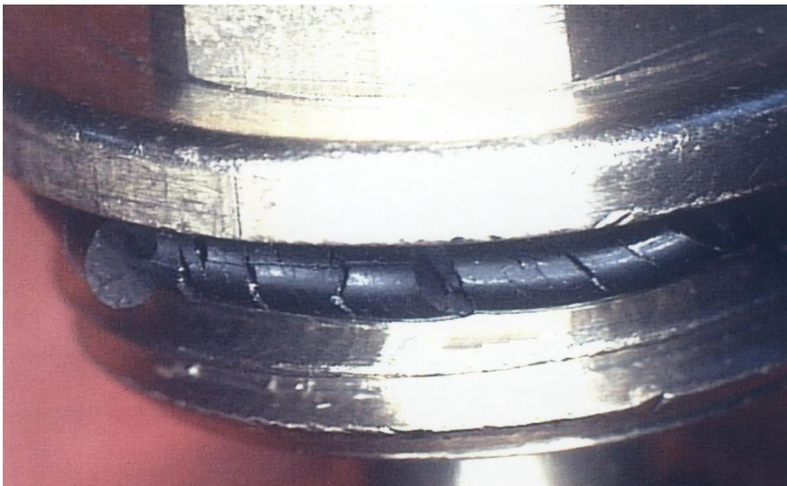
*Photo 5: Ozone splits on an assembled o-ring on sub component following several weeks in storage without light and air protection.*
