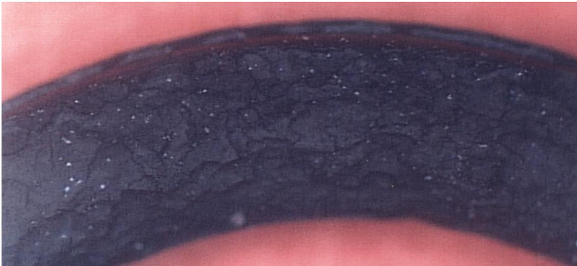
***Photo 13: Damage from explosive decompression of air.***
